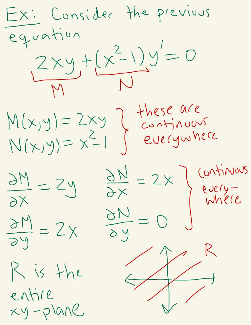
And,  $\frac{\partial M}{\partial y} = 2x = \frac{\partial N}{\partial x}$ Thus, 2xy + (x - 1)y = 0is exact. That is, there Will exist f with  $\partial f = M \& \partial f = N$
