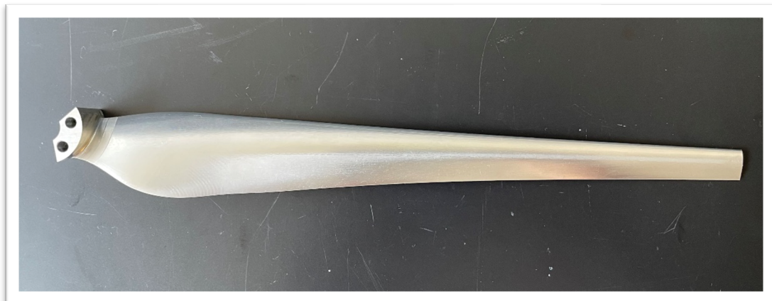
Figure 4 – 1/4 th Scale Aluminum Turbine Blade
