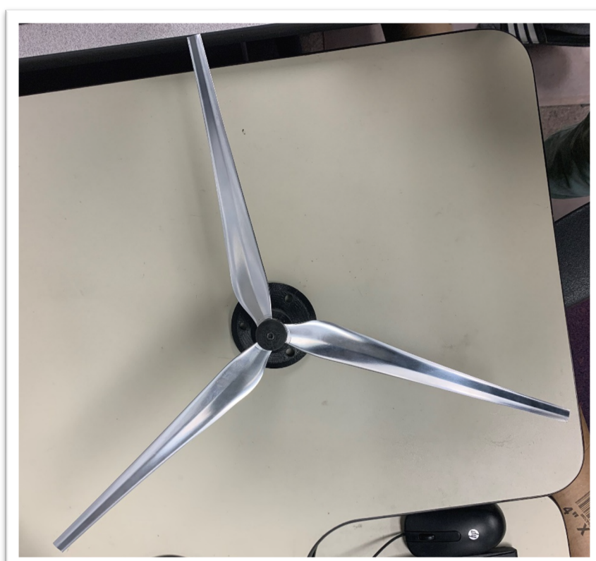
Figure 8 – 1/4 th scale turbine blades and hub
