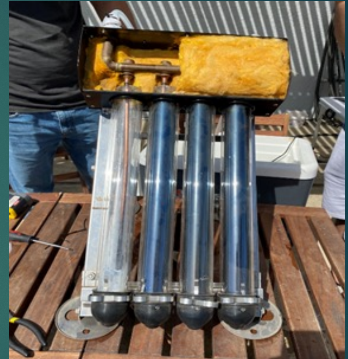
Evacuated tube Solar Hot water system
