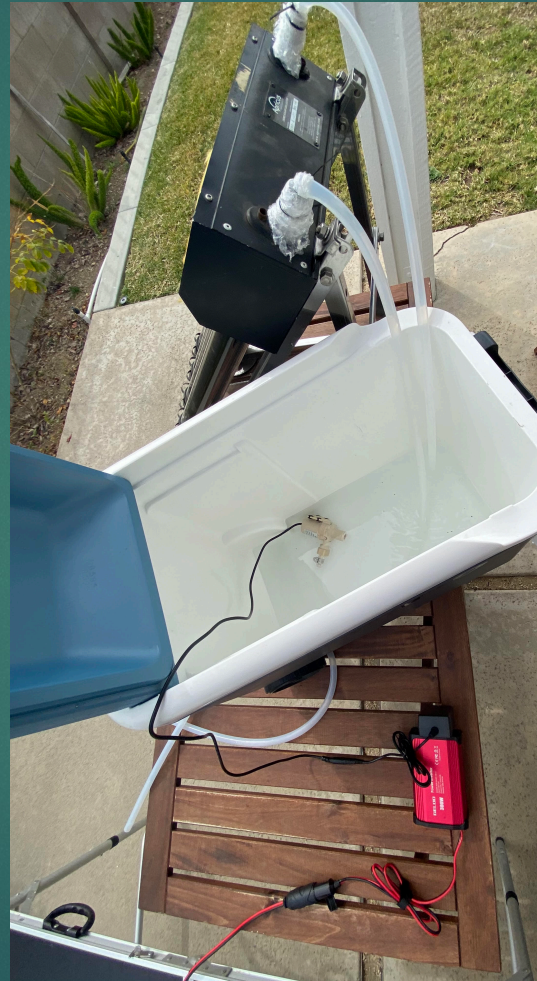
Water pump inside insulated cooler (1 gallon Water)
