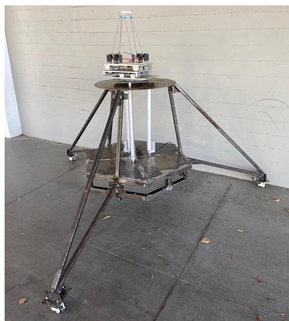
Frame under bending load (225 lb)
